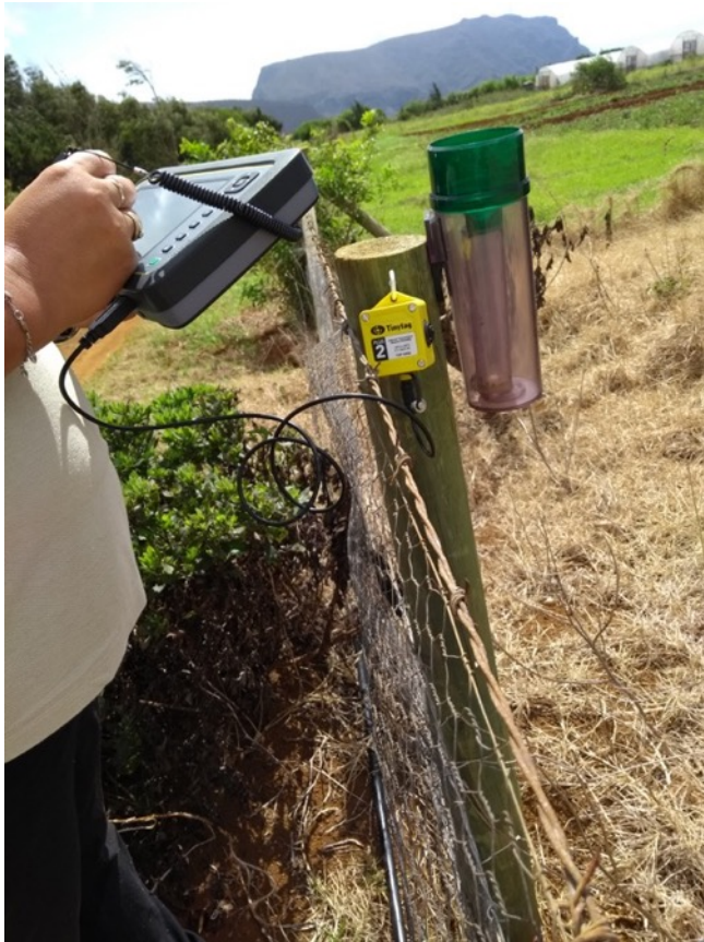
Source: ANRD, Saint Helena Government. Installing Temperature and Humidity Loggers
